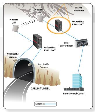
Additional switch-camera installations of similar configurations near Elko are also routed to the server room, which sends all of the information to the DOT control center in Reno.
